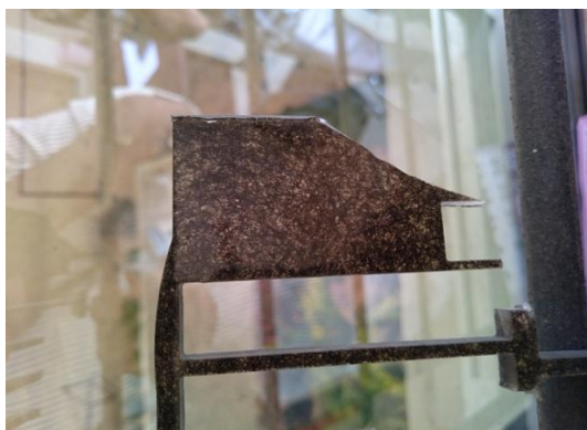
Fig. 2. Explores the composite which comprises 20% natural fiber which is used in the present investigation
