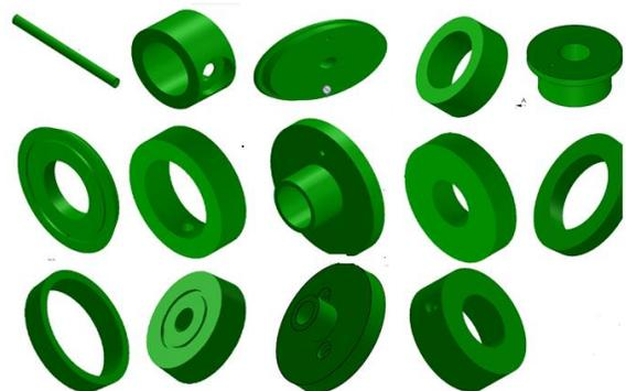
Fig. 3. 3D Part Diagrams for Welding Fixture
