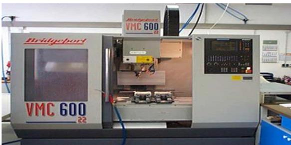
Fig 1. Vertical Milling Machine
